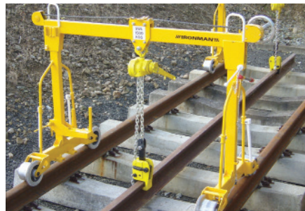
Typical application shots above showing a CR1000 in use with a Yale D85 Pul-lift and an 'Ironman' or left attached to YaleErgo 360 Ratchet Lever Hoist
